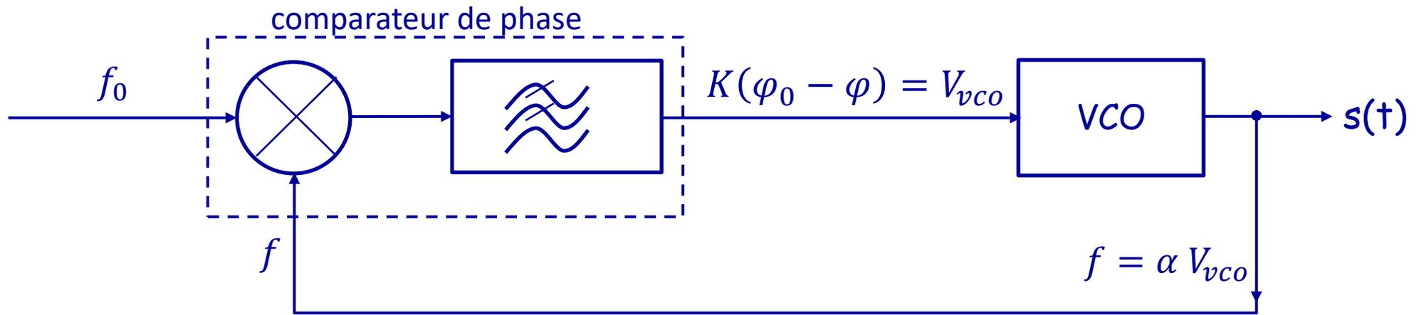
Si  $f = f_0 \implies \Delta\varphi = cste \implies V_{vco} = cste \implies f \text{ reste } cste = f_0$  Boucle verrouillée
